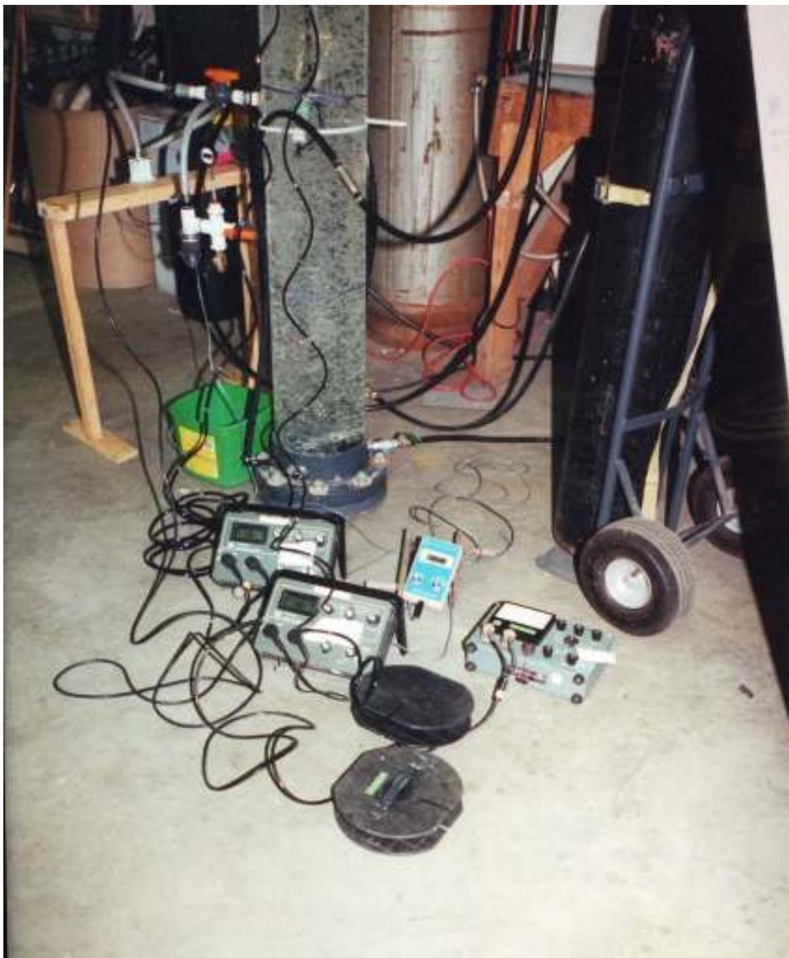
Picture 2. The three DO probes (2 YSI 58's, 1 YSI 57) are in the foreground. Column was being stripped with nitrogen when the picture was taken.
