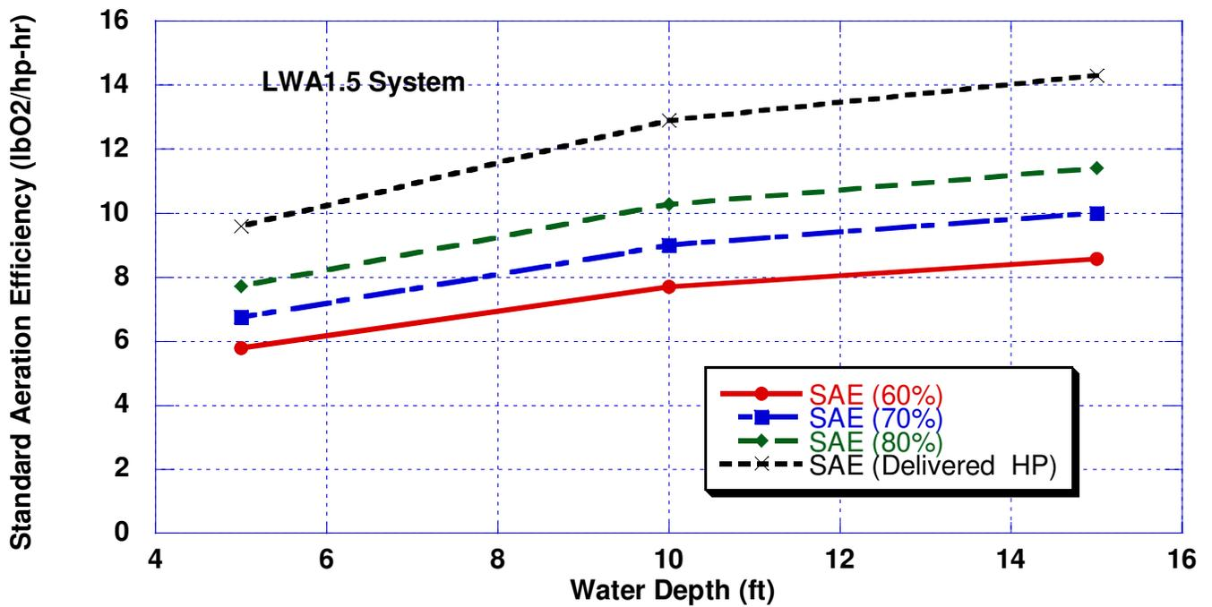
Figure 6. Standard aeration efficiency as a function of water depth and blower/motor efficiency for the LWA1.5 system (top)
