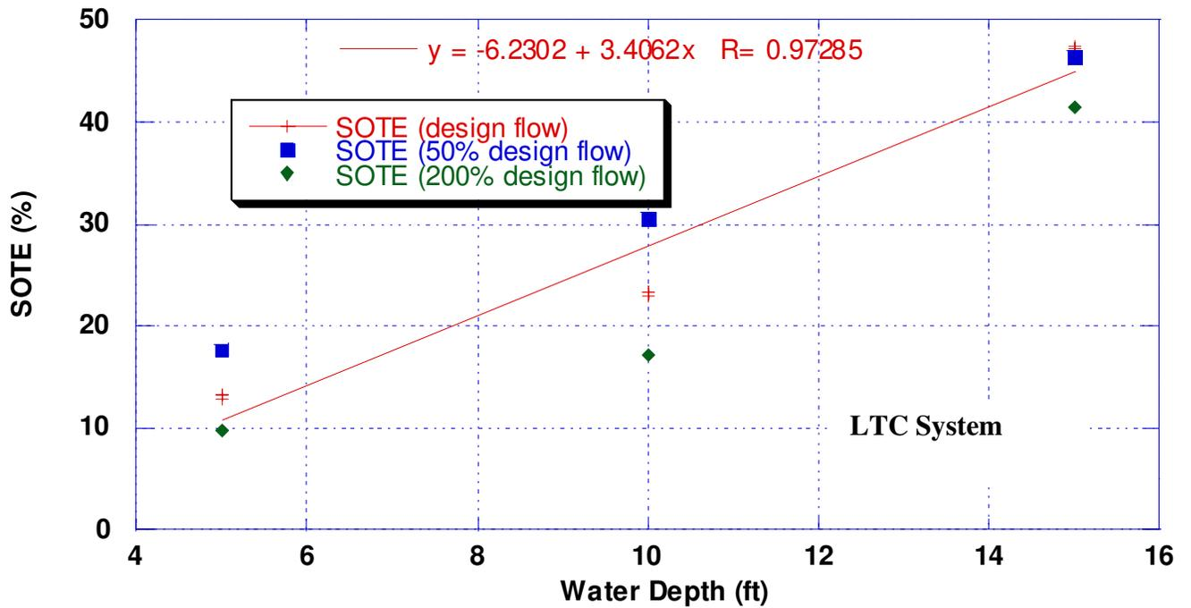
Figure 4 shows the SOTE for LTC tubing. The middle line (+ symbols) is the test result at the design flow rate. The diamonds and squares are results at the high (200% of design) and low (50% of design) airflow rates. As expected the efficiency at the lower airflow rate increased and decreased at the higher airflow rate. 15-foot depths do not follow the pattern. This is similar to the increased variability in the LWA1.5 test, and will be discussed later.
