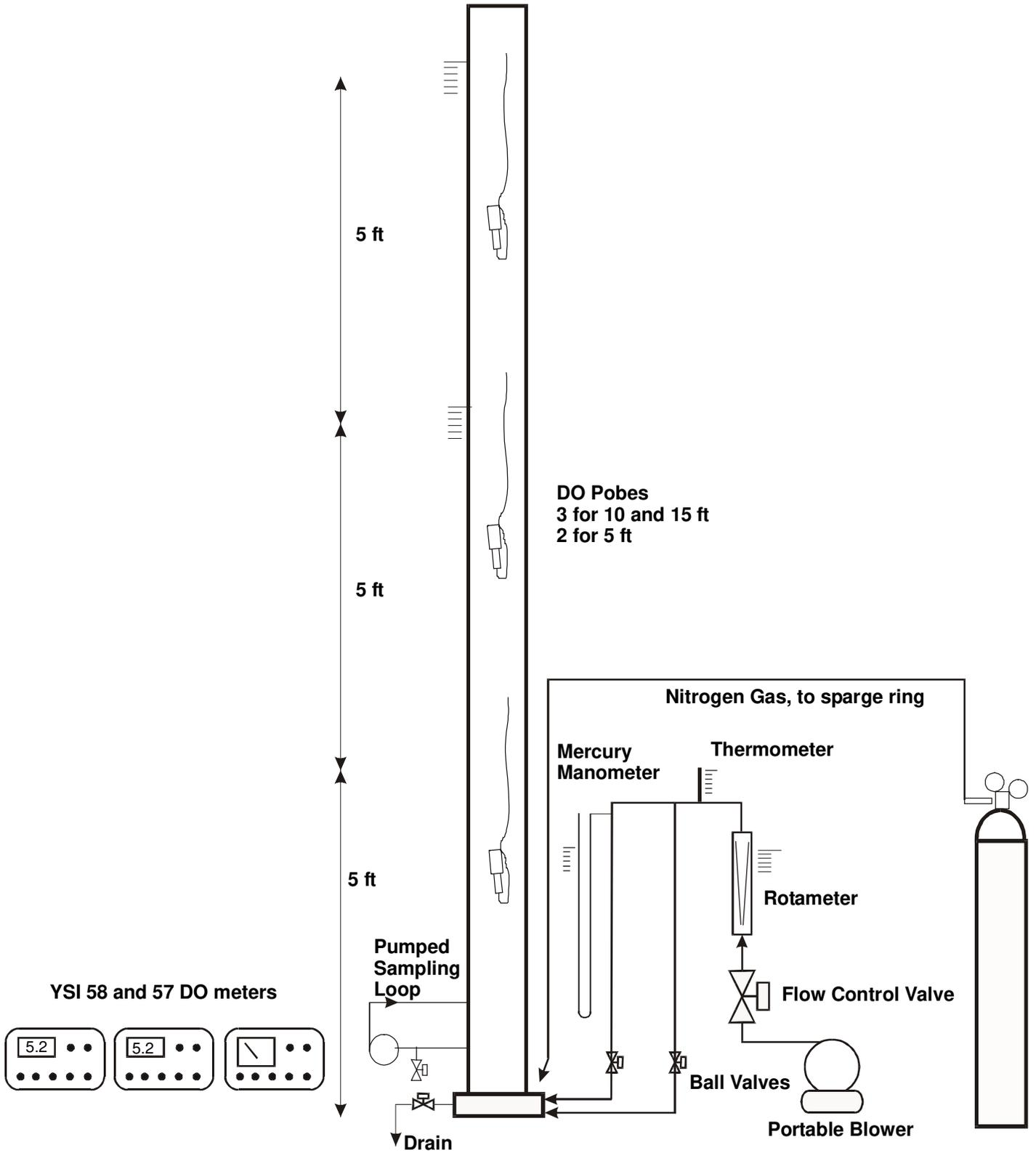
Figure 1. Test Column (8.75 inch ID) Schematic Diagram, showing DO meters and measuring instruments.
