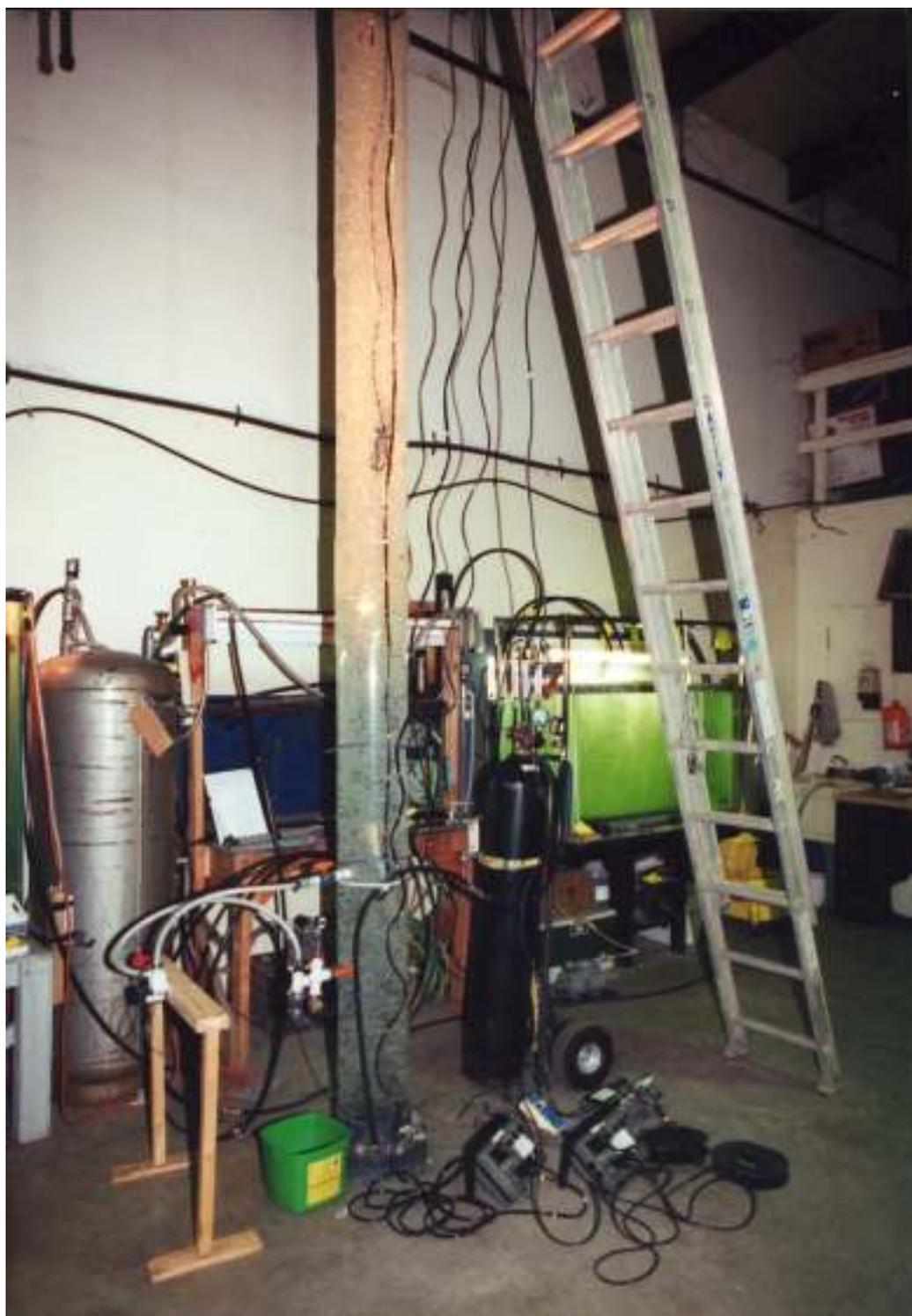
Picture 1. The column is in the center of the picture with the DO probes, nitrogen cylinder (black), and ladder clearly visible. The other tank, green aquarium and equipment were not part of the test.
