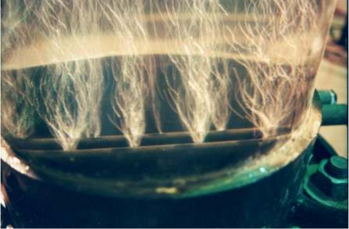
Picture 5. This picture, taken at slow shutter speed, shows the air release and bubble trajectories. Both LWA 1.5 and LTC tubing were operating during the picture. (Picture supplied by John Hinde).
