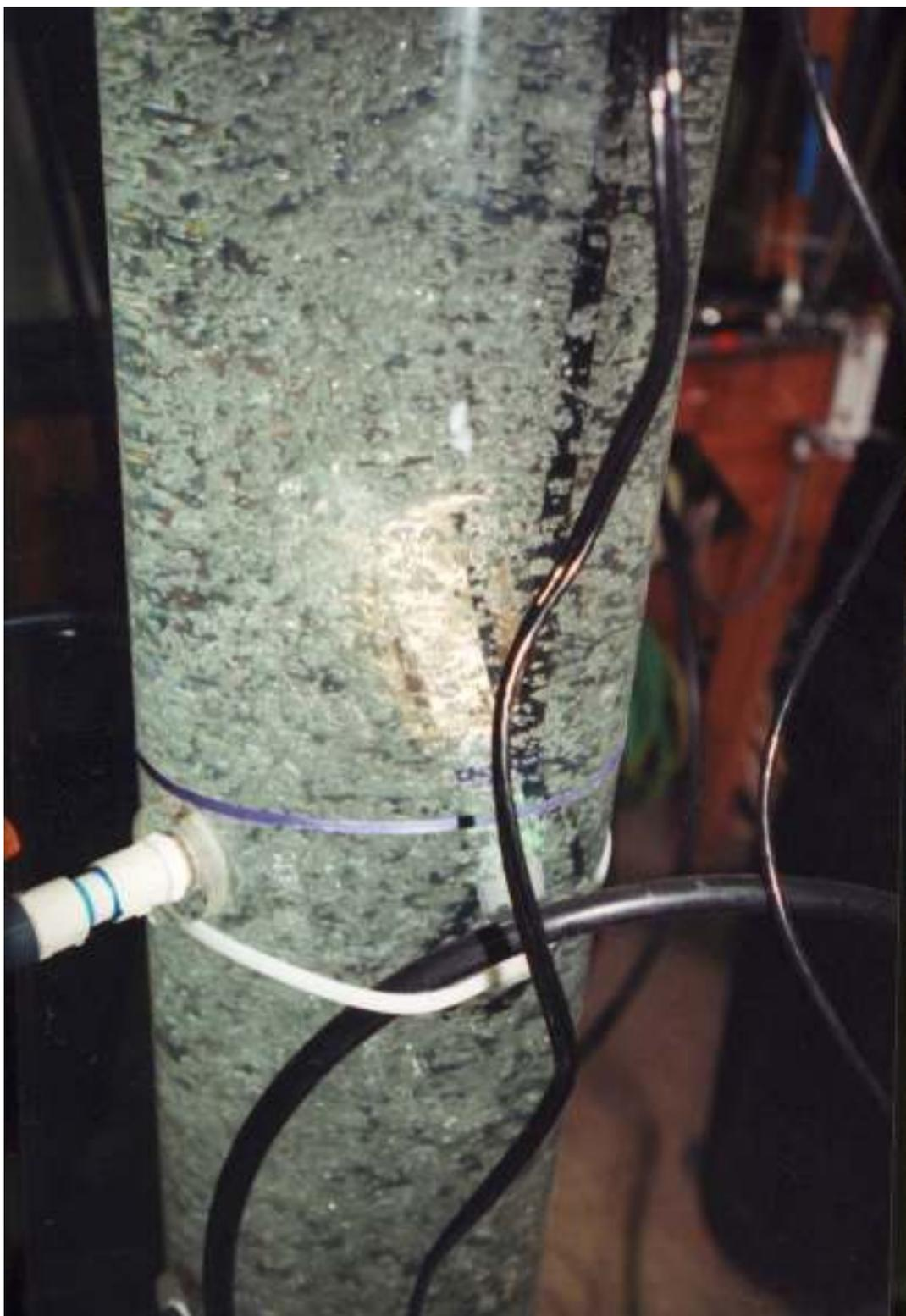
Picture 3. A large volume of nitrogen was used to strip the DO. A probe is visible behind the bubble swarm.
