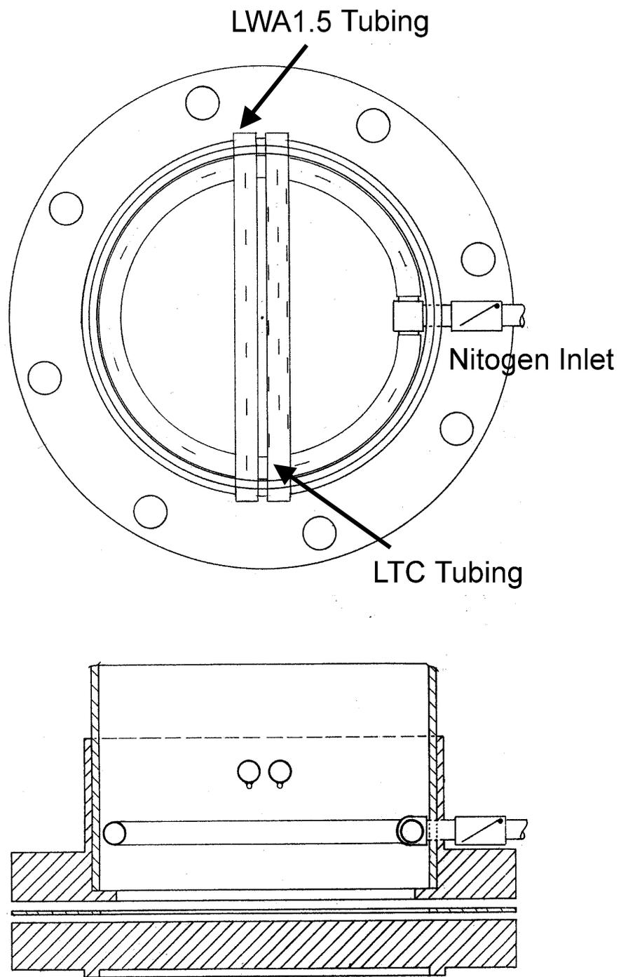
Figure 2. Details of the air diffusion tubing (drawing supplied by John Hinde)
