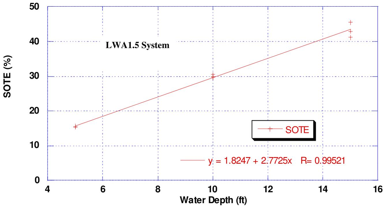
Figure 3: Standard Oxygen Transfer Efficiency (SOTE) versus Water Depth for the LWA1.5 system at the standard airflow rate (**above**).
