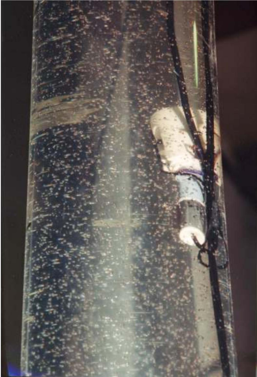
Picture 4. This picture shows the column and DO probe during aeration. The bubble density is much less than during nitrogen stripping.
