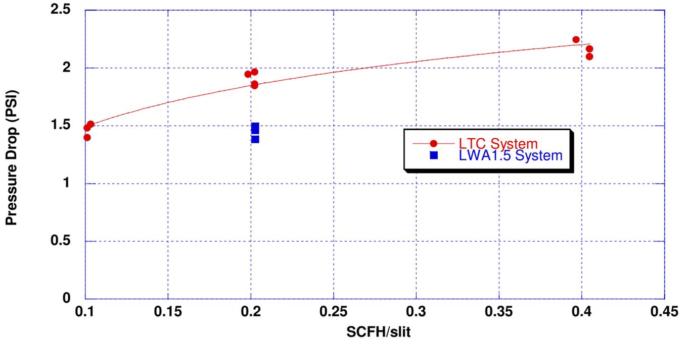
Figure 5. Pressure drop versus airflow per slit
